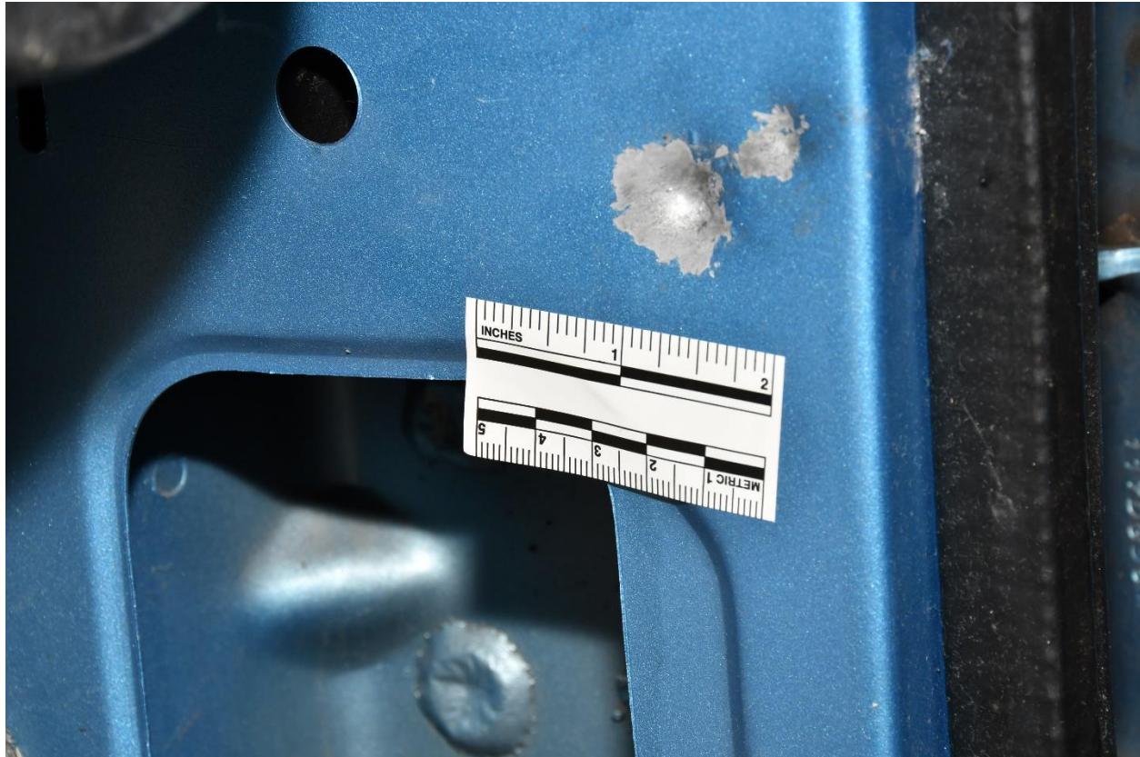
Figure #63 – Suspected ballistic impact to vehicle frame behind passenger floor column panel
