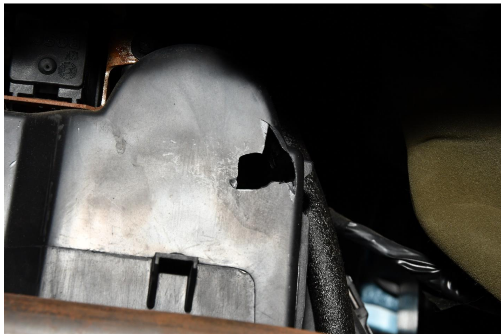
Figure #52 – Suspected ballistic impact to wall behind glovebox
