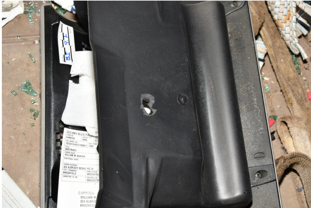
Figure #51 – Suspected ballistic impact to exterior back of glovebox
