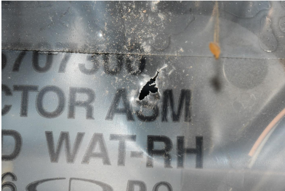
Figure #60 – Suspected ballistic impact to plastic behind passenger door panel
