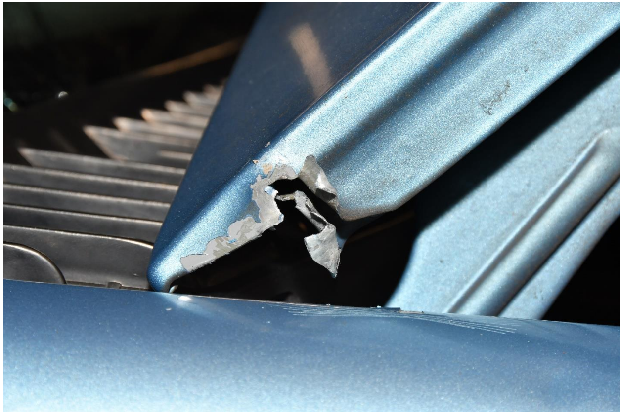
Figure #45 – Ballistic impact to passenger side hood
