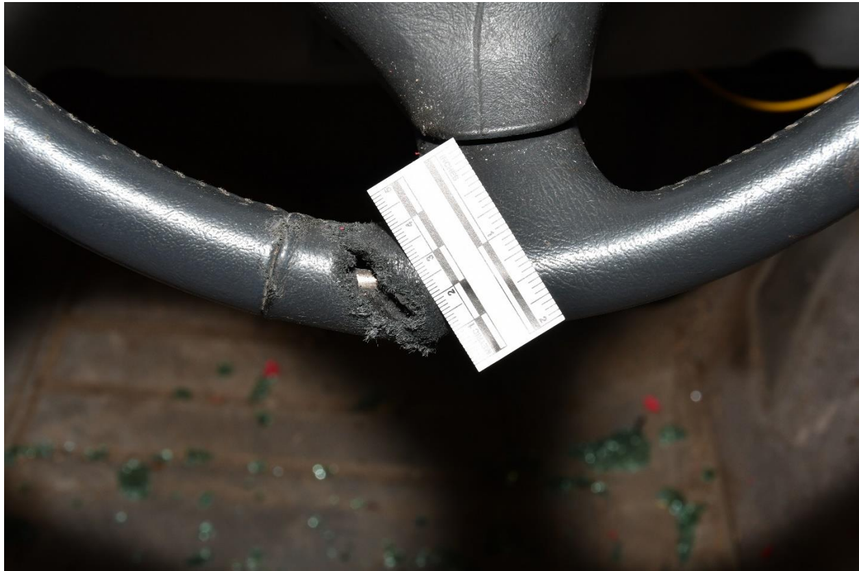
Figure #64 – Suspected ballistic impact to steering wheel
