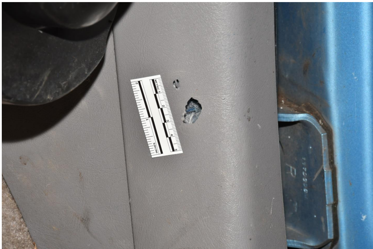
Figure #62 – Suspected ballistic impact to passenger floor column panel
