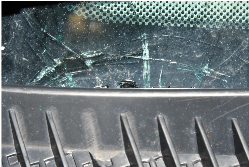
Figure #43 – Ballistic impact to lower passenger side windshield
