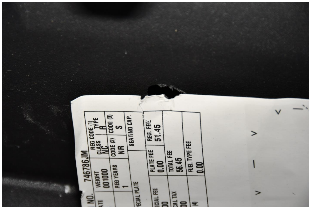
Figure #50 – Suspected ballistic impact to interior back of glovebox
