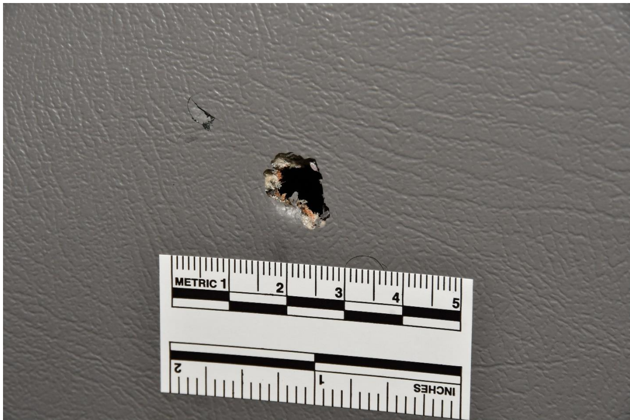
Figure #59 – Suspected ballistic impact, interior passenger door
