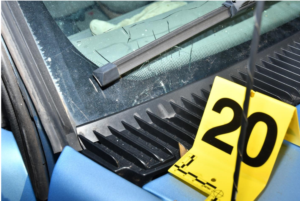
Figure #26 – Passenger side lower windshield broken
