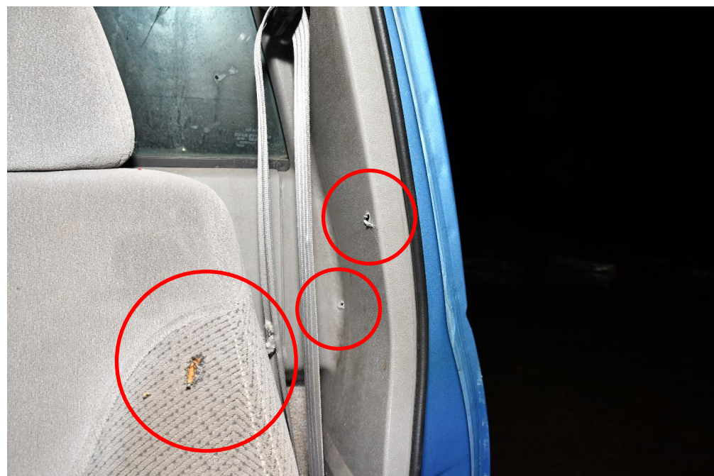
Figure #21 – Suspected ballistic impacts perforating B-pillar, driver seatbelt & seat
