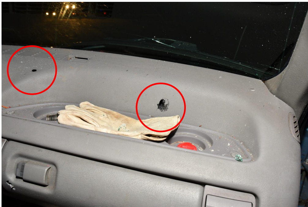
Figure #25 – Suspected ballistic impact perforating passenger side dashboard
