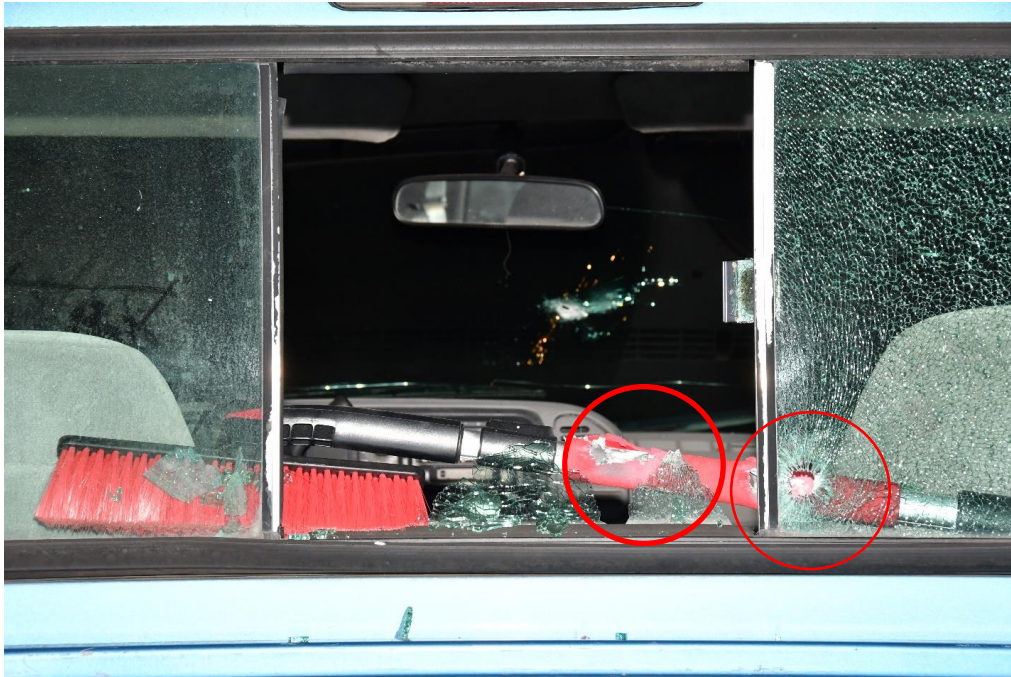
Figure #18 – Rear window of pickup truck with suspected ballistic impacts
