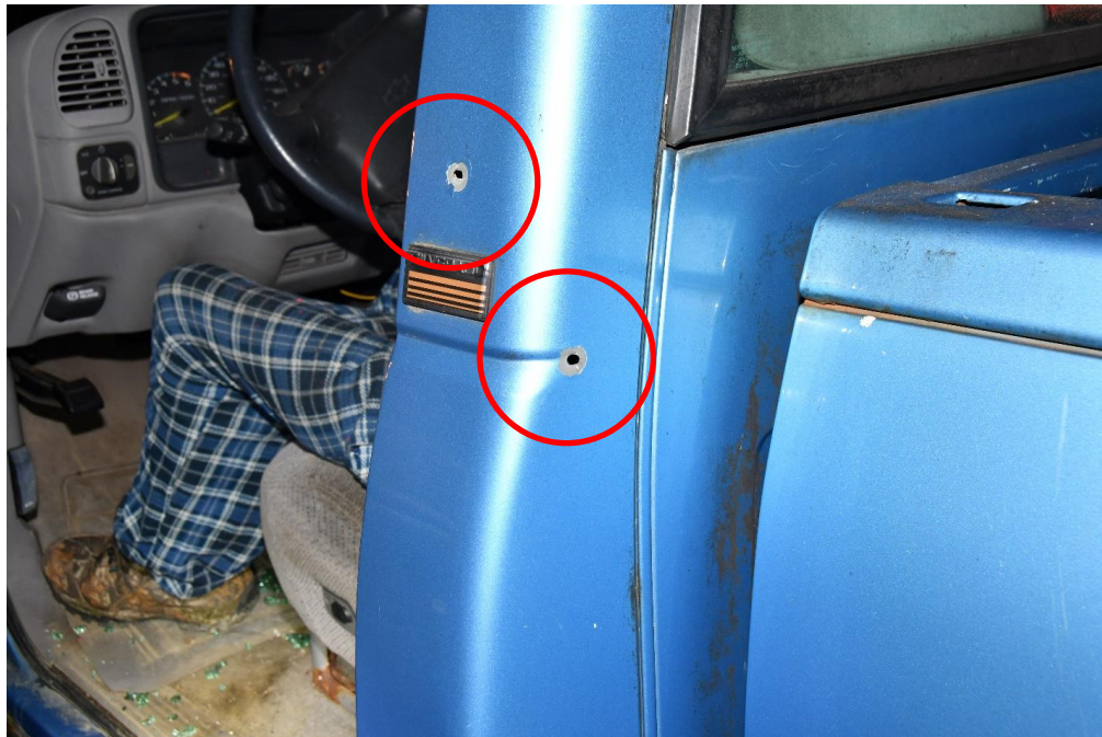
Figure #20 – Suspected ballistic impacts perforating B-pillar
