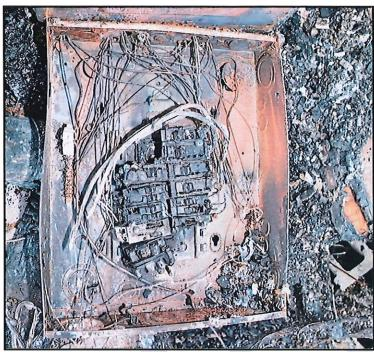
Figure 6- View of the main electrical distribution panel
