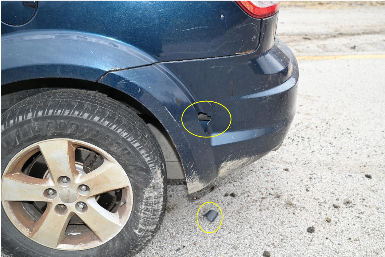
Damage on Dodge Journey's left rear bumper
