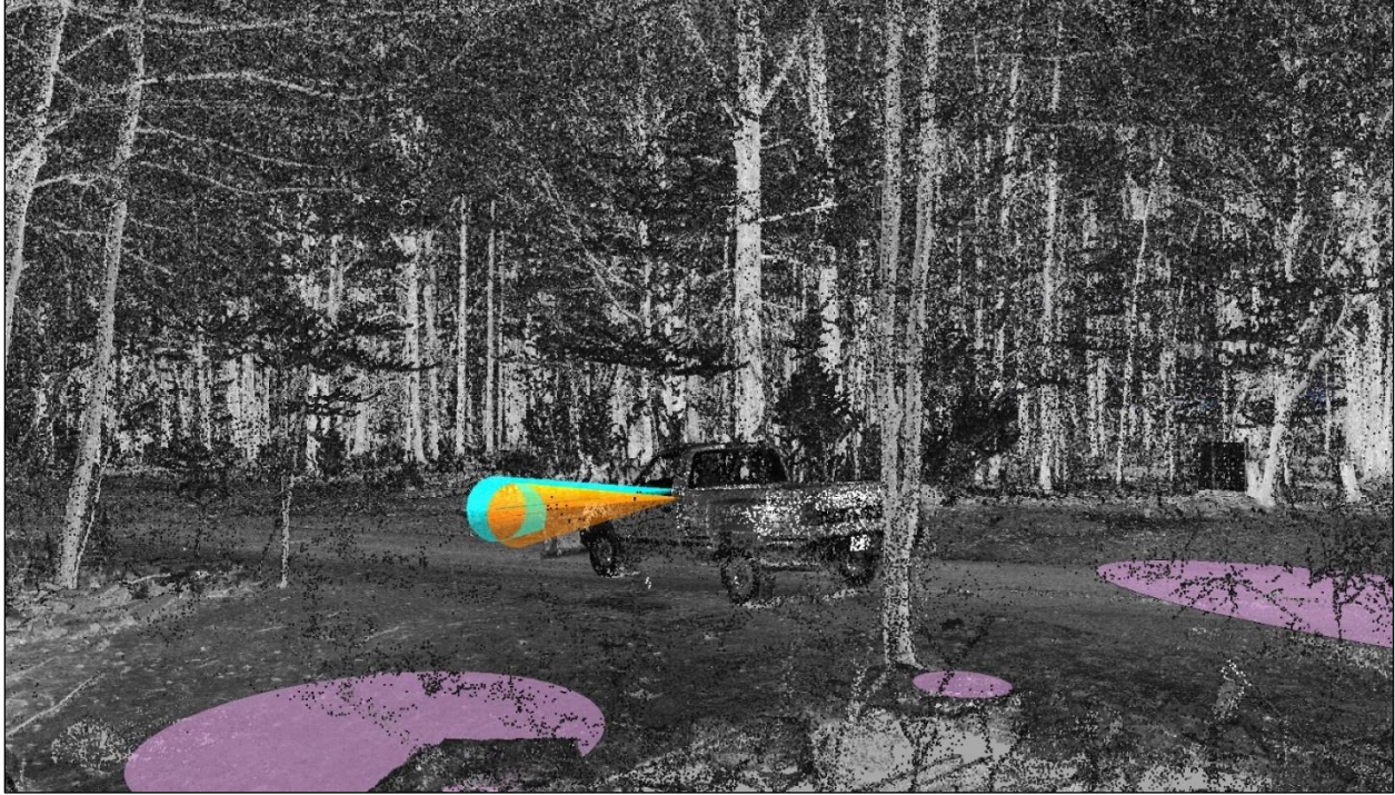
Trajectories 1 (teal) and 2 (orange) from a left rear perspective. Vehicle at final rest.
