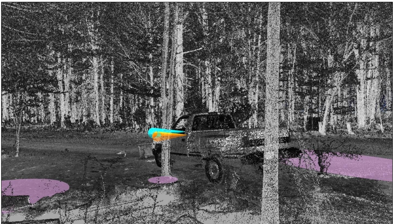
Trajectories 1 (teal) and 2 (orange) from a left rear perspective. Vehicle along path from start to final rest.
