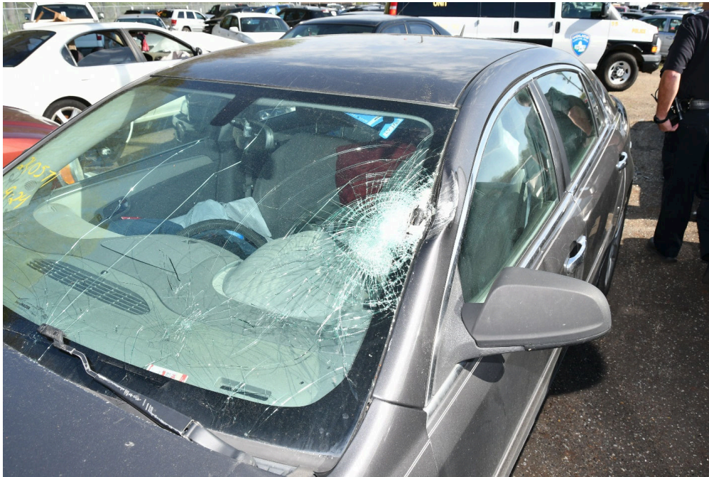
Figure #4 - Damaged windshield
