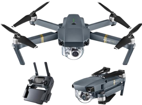
The DJI Mavic folds into a small size for stow and transport.
