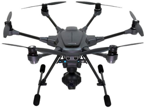
The YUNEEC Typhoon H is an example of a hexacopter with six rotors.
