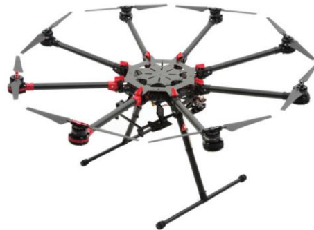
The DJI S1000 is a semi-custom octocopter known for having an impressive payload capacity for a multi-rotor and for its stability when used for photography.
