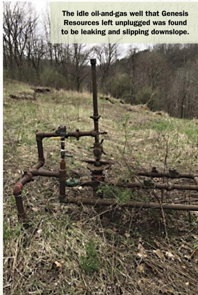
The idle oil-and-gas well that Genesis Resources left unplugged was found to be leaking and slipping downslope.
