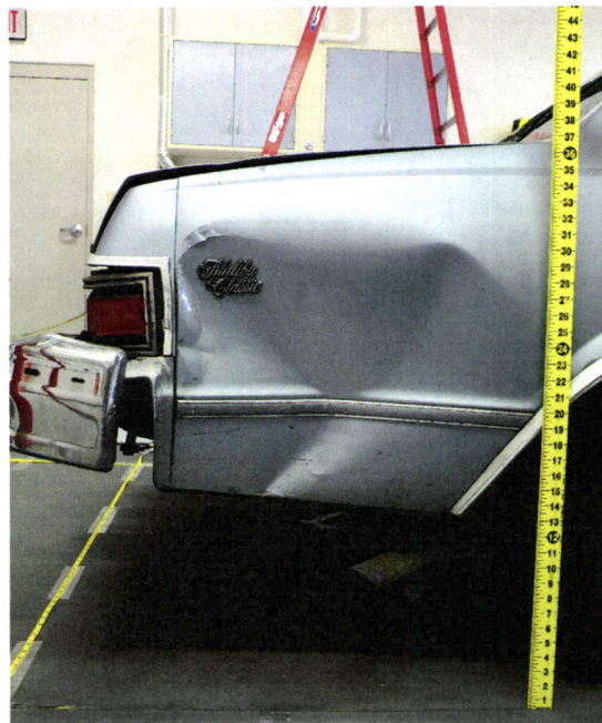
Figure 4 (pass. side quarter panel damage)
